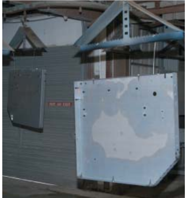
A laser-cut and press-brake-formed sheetmetal-cabinet component leaves the Metcam five-stage pretreatment line ready to enter the firm's three-booth conveyORIZED paint line.
